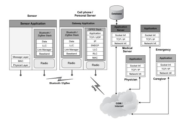
Figure 3: Mobile medical care system architecture and components
