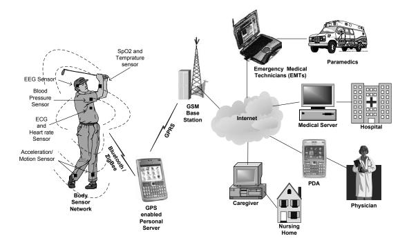
Figure 2: Wireless body sensor network for pervasive health monitoring
