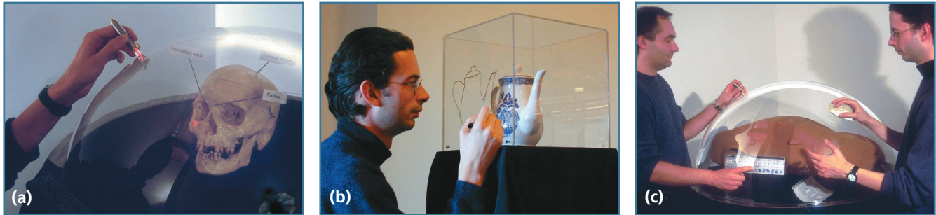
Figure 2. Volumetric-display mockups: (a) 2-foot diameter dome; (b) 1-foot cubic enclosure; (c) 4-foot large-scale dome. Developers place a variety of physical objects within the clear plastic enclosure to explore the affordances of volumetric displays that differ in size, form, and use.
