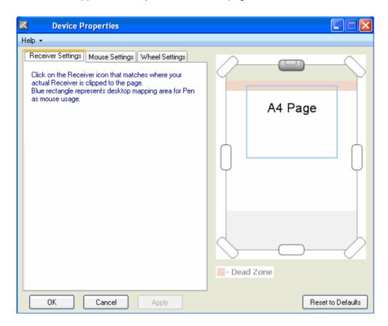
You can change this configuration by clicking on one of the placement markers on the Receiver Settings section. If for example, you click on the middle left marker, then Digital Pen&Mouse configures the Digital Pen's range with the understanding that the Receiver is attached to the right side of the page.
