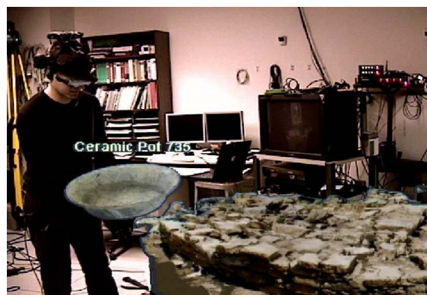
Figure 8. Our augmented reality visualization system. A user in our lab explores a full-size model of the site and selects one of the findings to examine in detail. This image is taken through a live, tracked, video see-through display.
