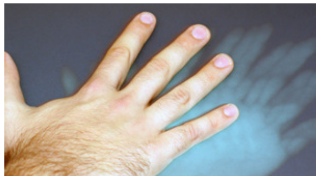
Figure 2. An early attempt to visualize input by displaying raw sensor data. This approach does not generalize across device types.
