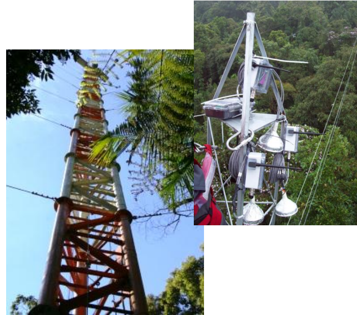
One of six towers equipped with sensors to measure temperature, water vapor, and solar radiation
