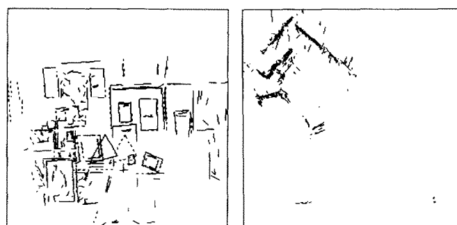
Figure 10. Superposition of two scenes with the result of EKF-AXIS using 105 line segment correspondences
