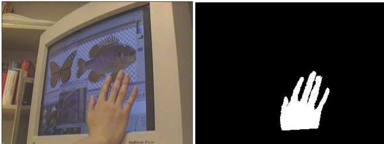
Figure 5: Segmentation result. Left image shows a picture of a hand on the screen. Indicator could be any finger of the hand. Right image shows the segmented hand. Note that the segmentation result is not affected by the complicated screen background
