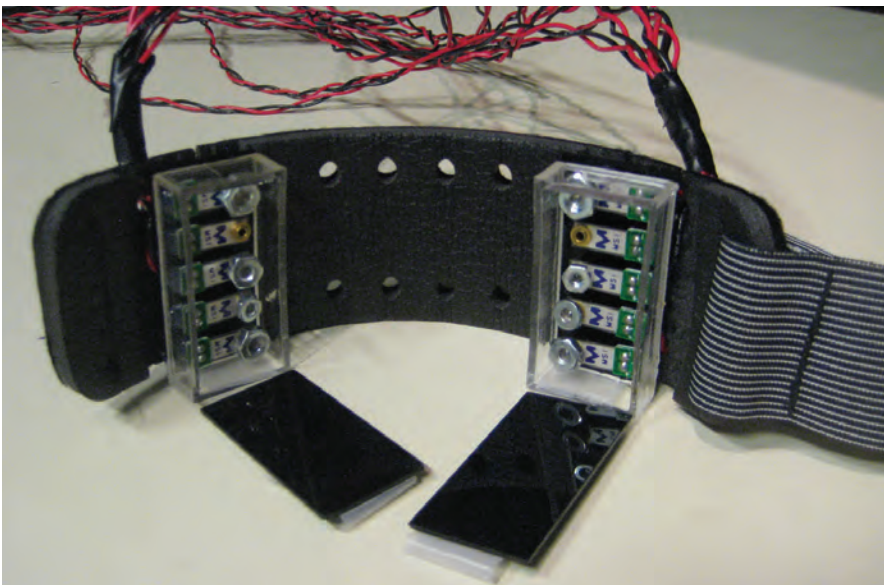
Figure 2: Our prototype features two arrays of sensing elements incorporated into an armband form factor. Each element is a cantilevered piezo film tuned to respond to a different, narrow, low-frequency band of the acoustic spectrum.
