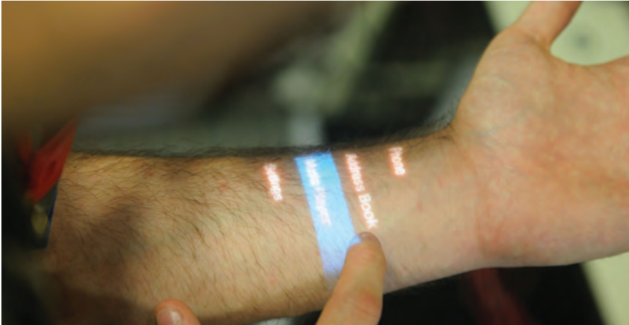
Figure 3: Augmented with a pico-projector, our sensing armband allows interactive elements to be rendered on the skin, potentially enabling a new class of mobile computing experiences
