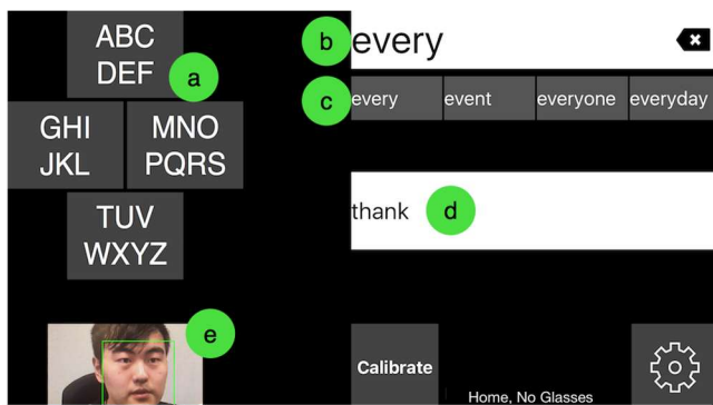
Figure 7. Interpreter interface: (a) four-key keyboard; (b) the word input box shows top prediction of characters entered in the current sequence; (c) top four word predictions; (d) the sentence box shows prior words in the communication; (e) camera preview with a green face detection box.
