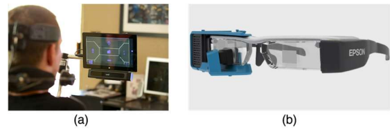
Figure 3. High-tech gaze recognition solutions: (a) Tobii Dynavox eye-tracking computer [28]; (b) EyeSpeak eye-tracking glasses [18].
