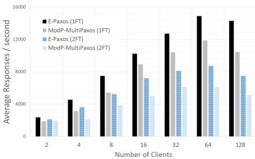
Fig. 15. Performance of ModP HashTable using Multi-Paxos (MP) is comparable with an open source baseline implementation (mean over 60s close-loop client runs).
