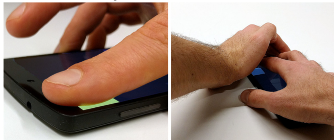
Figure 1. Our Android app captures oximetry reflections from the finger using the display as an illuminant in solely the red and green spectrum (thus appearing yellow). This produces significantly more accurate oximetry values than when using the rear camera and the flash for illumination.
