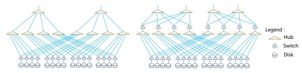
Fig. 2: Interconnect fabric. The left design uses hubs and switches to form two full trees to connect disks to two hosts, while the right design places switches at a higher level of the tree to allow better throughput.
