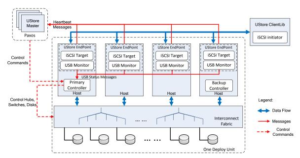
Fig. 3: The software architecture of UStore. The interconnect fabric uses the topology elaborated in § III, upper layer services interact with hosts directly for data flow after retrieving metadata from the Master.
