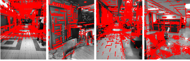
Figure 3. Examples of verified query poses. We evaluated the quality of the reference camera poses both visually and quantitatively, as described in section 3. Red dots are the database 3D points projected onto a query image using its estimated pose.
