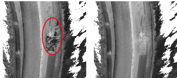
Fig. 10: Example of reconstructed 3D points (left) without and (right) with moving object detection for South Buona Vista .
