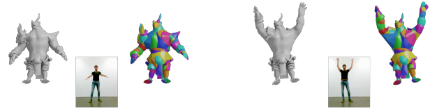
Fig. 12. The user controls the original mesh via a Kinect and a precomputed approximate convex decomposition is transferred in real-time to the novel frames.
