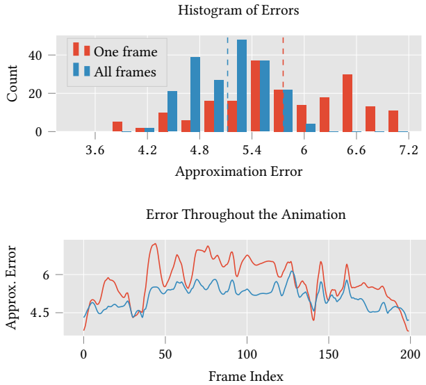
Fig. 9. Difference between the decomposition of an animated mesh into 16 parts computed from only the first frame of the animation (red) and all frames (blue). The lower plot shows the approximation error throughout the 200 frames of the animation. The upper plot shows the histograms of those approximation errors. One can see that the decomposition computed from only the first frame “overfits” that frame and produces a low approximation error only for this and similar frames. The decomposition computed from all frames on the other hand has lower mean approximation error as well as a lower standard deviation in those errors.
