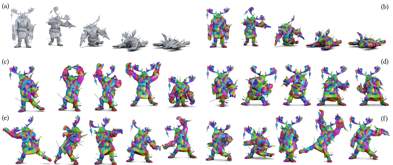
Fig. 7. Temporally coherent approximate convex decomposition and transfer for an animated mesh. a) Input animation, b) Approximate Convex Decomposition, c) d) e) f) Transfers to new previously unseen animations. More transfer results in the teaser figure.
