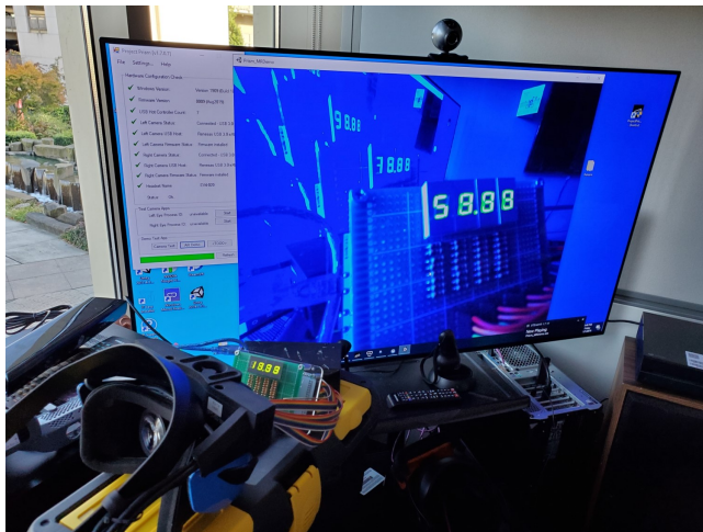
Figure 6: Setup for the alternate hardware instrumentation-based measurement method. The screen shows a mirror of the actual HMD display at 120Hz. While the real Arduino Clock is standing right in front of the cameras. This image is taken directly from the measurement camera.
