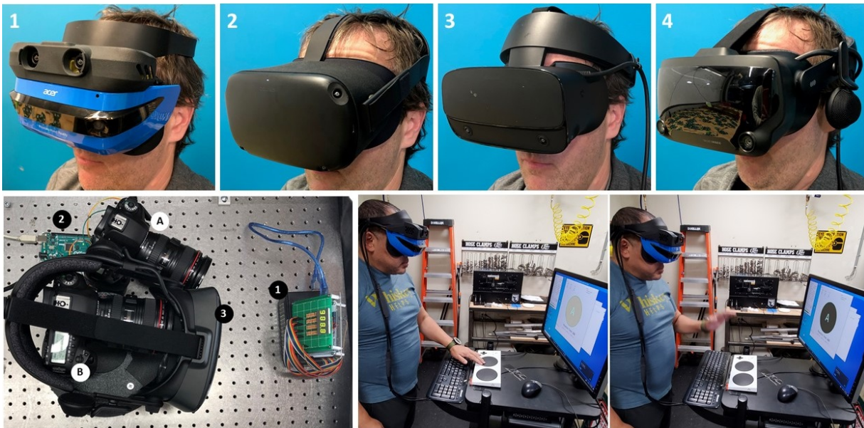
Figure 1: Latency was tested both through a hardware instrumentation-based measurement (bottom left) and the new cognitive latency technique (bottom right) on four different devices. The first device, Prism, was an ad-hoc system that attached a pair of colour cameras to an Acer Windows Mixed Reality device (1 top left). This system aimed at providing a top end video see-through quality. We also tested Oculus Quest (2), Oculus Rift S (3) and the Valve Index (4). On the Bottom Left, hardware instrumentation-based measurement setup. Cameras (A and B) are synchronized to capture at the exact same time by the board (2). While (1) is a clock running at sub-millisecond accuracy. The clock for camera (B) is seen by the HMD (3), which displays the video see-through. The scene was kept well illuminated to reduce automatic exposure time problems of the HMD cameras. On the Bottom Right, a participant performing the rapid decision making task while wearing a see-through VR headset.
