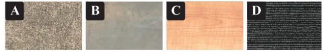
Figure 9. Sample material tiles used to record texture models and sound. A) Concrete, B) metal (aluminum), C) hardwood tile, and D) short carpet.
