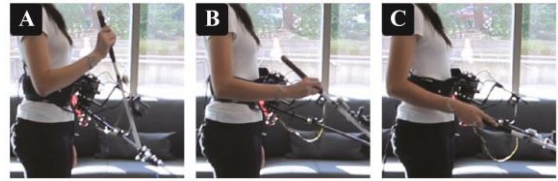
Figure 3. A) Traditional cane grip centered-high, B) pencil cane grip centered-low, C) standard cane grip centered-low.
