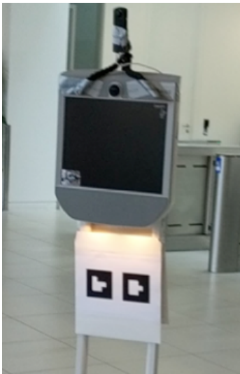
Figure 7: The robot with the marker pattern (bottom) and 360° camera (top).
