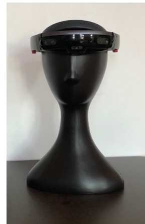
Figure 1: The Wearable Headset Prototype. It consists of an adjustable “headband” with one forward-facing camera, and three peripheral cameras. It also has bone-conducting earphones to provide spatialized audio. A small battery pack is included to the rear of the headset.
