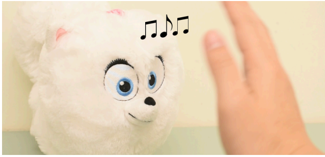
Figure 9 Interactive plush toy for children. Waving the hand near the dog triggers a greeting sound. Touching its head plays a prompting sound.
