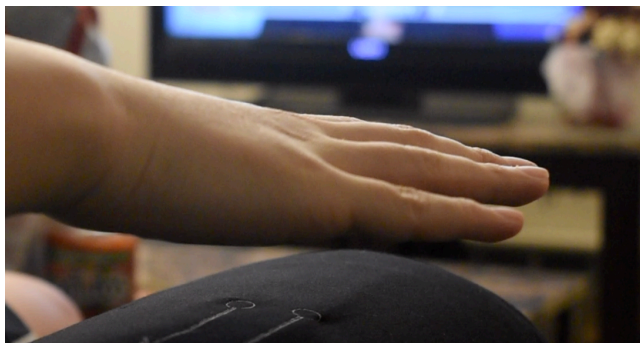
Figure 6. Interactive furniture. A touchless remote control on the armrest of a sofa.
