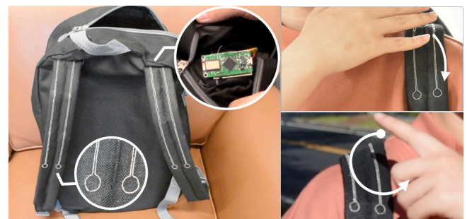
Figure 8. The straps of a backpack are modified by covering the sensors, which also allows for dual gestural input.
