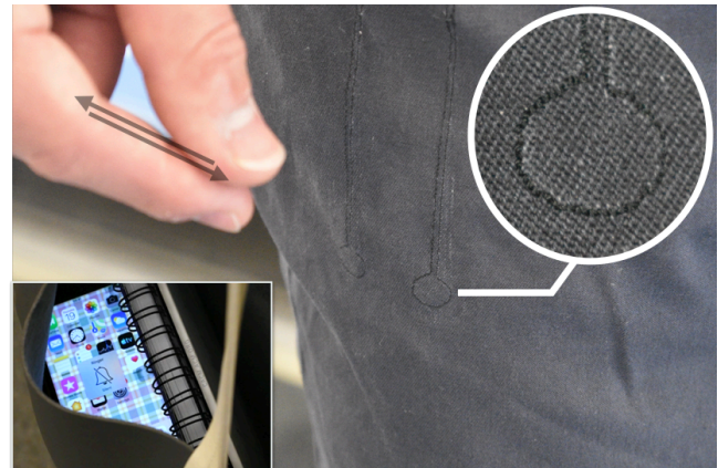
Figure 1. Fabriccio enables touchless gesture sensing on interactive fabric. For example, by embedding Fabriccio into pants, a user can perform subtle arms-down gestures to interact with a phone.
