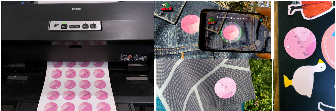
Figure 1. (left) EcoPatches can be printed by a maker with an inkjet printer and chemicals that can be purchased online. (right) EcoPatches can be read at a glance or interpreted with a companion smartphone app.
