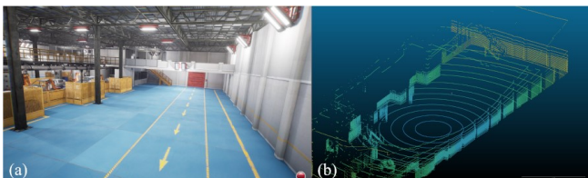
Fig. 9: Extracted LiDAR points. (a) Virtual environment. (b) 32-line LiDAR points.
