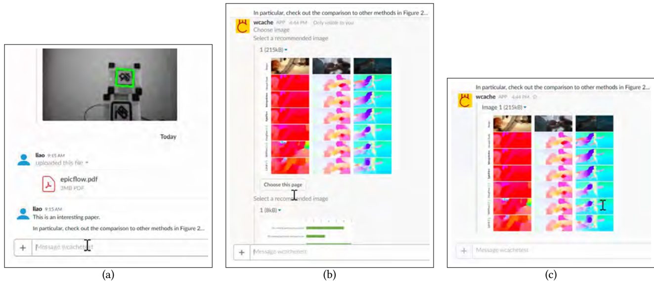
Figure 1: (a) Sharing documents in multimedia chat tools tends to hide critical content. Using online document analysis tools, users can more easily call out digital artifacts that can serve as conversational props. (b) An automated tool automatically identifies two candidates matching the reference “Figure 2” in the user’s comment. (c) The user clicks a button to manually disambiguate the reference and the figure is injected into the chat.
