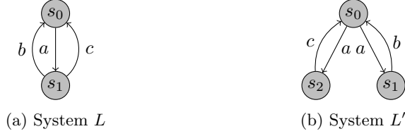
Figure 3.3: Counter-example to converse of Theorem 3.1 [Pg. 34]: Lang(L) \subseteq Lang(L') , but L' does not simulate L
