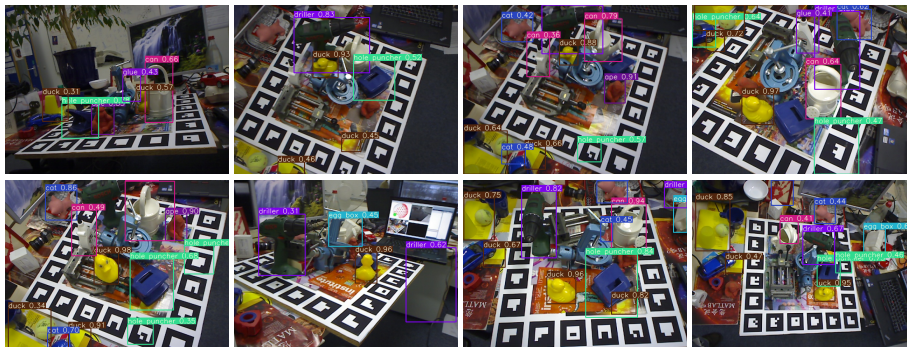
Fig. 4. Sample detections on real images from LM-O dataset, using a network trained on synthetic images generated by Arnold renderer, which is optimized with AutoSimulate using real-world images.
