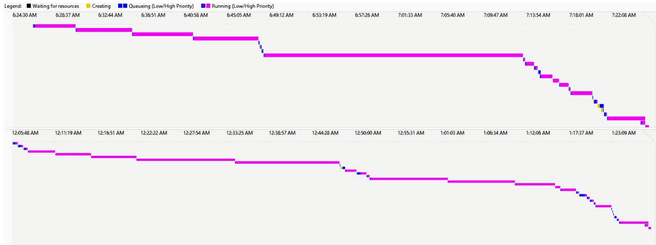
Figure 2: The critical path of execution for two occurrences of the same job. The top one completed in 57 mins, while the bottom one took 88 mins to complete. Each line of each occurrence corresponds to a job stage’s start/finish time. Just by looking at this visualization tool, one might think that the top job is the errant job (due to some long stages), while in fact the bottom one is the one diverging from the normal behavior.
