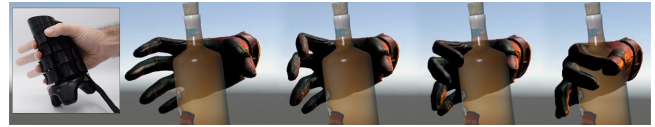
Figure 11: As the user touches the controller (left), a quick animation of their virtual hand closing its fingers around the virtual object is triggered (right). A similar animation of the virtual hand releasing the object is displayed when the user releases their grasp.
