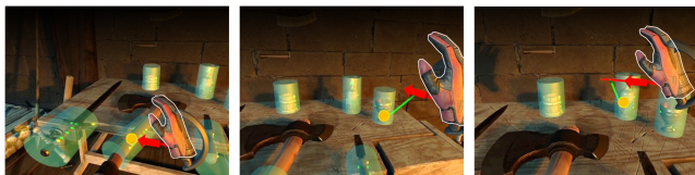
Figure 10: Object prediction uses a temporally smoothed hand velocity vector (red arrow) to find the nearest graspable object to this ray (marked by a yellow dot).
