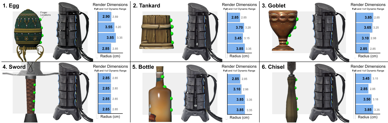
Figure 7: Six objects tested in the user study. Each virtual object is shown alongside its corresponding rendered shape on X-Rings as well as the physically rendered dimension of each layer, as computed according to the Shape Sampling protocol detailed in Section 3.7. Dimensions for both full and half dynamic range conditions are given. Green circles on each virtual object indicate the grasp point for each finger.
