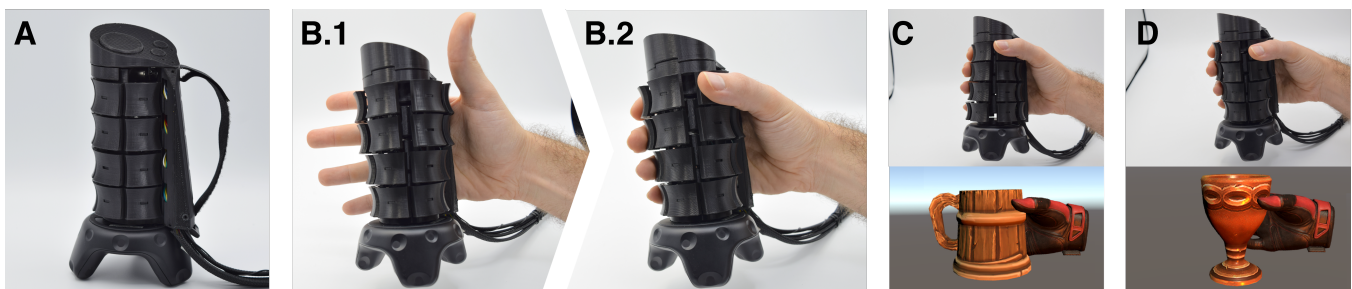
Figure 1: X-Rings (A) is a 360° shape display designed to support grasping. The device is hand-mounted (B.1), allowing the fingers to grasp and release rendered objects freely (B.2). Four expanding layers enable rendering of many virtual objects, such as a tankard (C) and goblet (D).
