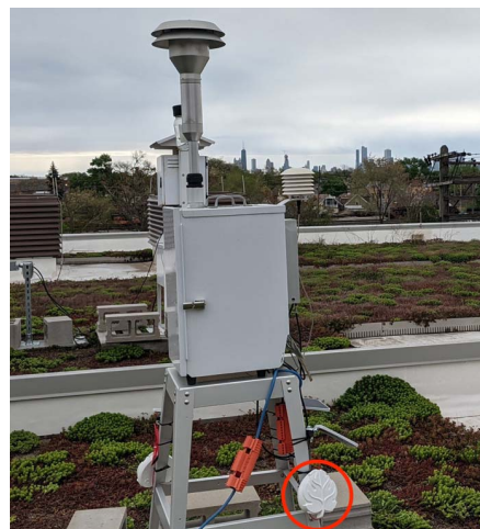
Figure 4: Three Eclipse devices were co-located with air pollution monitoring equipment at each of three EPA sites in the city of Chicago throughout the deployment to enable the evaluation of accuracy and the development of data calibration models.
