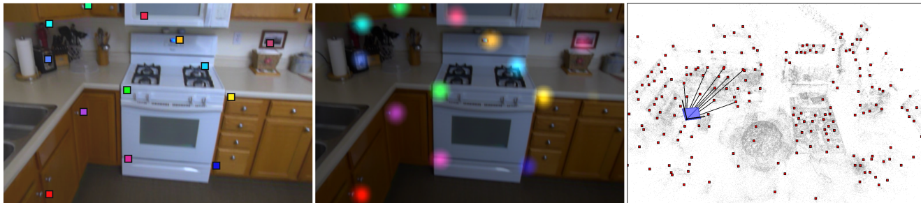
Figure 1. We present a new method to recognize scene-specific scene landmarks to localize a camera, which preserves privacy and achieves high accuracy. [Left] Scene landmark detections in a query image obtained from a heatmap-based CNN architecture. [Middle] A visualization of the predicted heatmap scores. [Right] The 3D scene landmarks (in red) and the estimated camera pose (in blue) are shown over the 3D point cloud (in gray). The 3D point cloud is shown only for the purpose of visualization.
