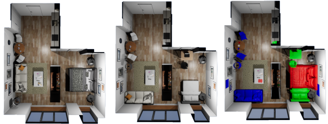
Fig. 4: Flat dataset. Run 1 (left), run 2 (center), and changes (right), showing new (green), removed (red), and modified (blue) objects.
