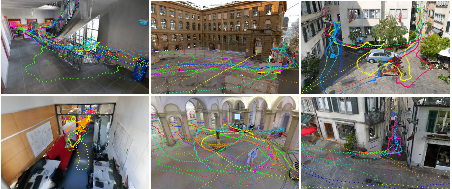
Fig. 2. The locations feature diverse indoor and outdoor spaces. High-quality meshes, obtained from lidar, are registered with numerous AR sequences, each shown here as a different color.
