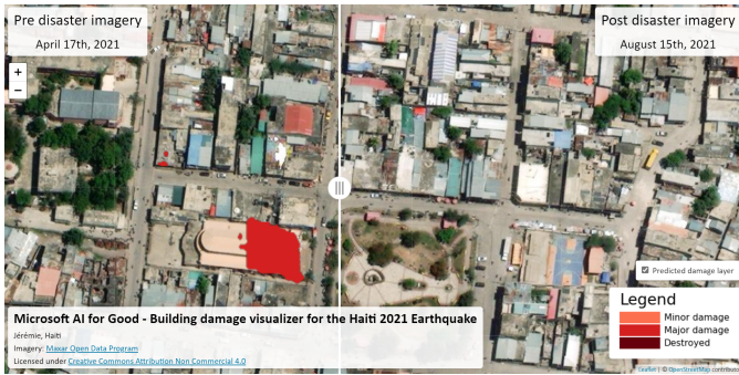
Fig. 6. Screenshot of the building damage visualizer instance for the August, 2021 Haiti Earthquakes. The left side of the map interface shows the pre-disaster imagery while the right side shows the post-disaster imagery. The slider in the middle of the interface allows a user to switch between the pre- and post-disaster layers to quickly see the difference in the imagery. Finally, the building damage predictions are shown as polygons with varying shades of red corresponding to increasing damage. The visibility of these predictions can be toggled in the interface so that a user can see the underlying imagery.
