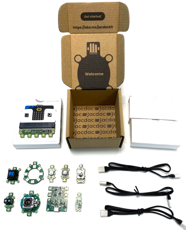
Fig. 12. A Jaccac hardware kit for the micro:bit V2, as used by hackathon participants.
