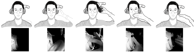
Figure 5: Selected gestures we used for our prototype system. The bottom shows LiDAR images of those gestures. (From left: default mode, cupping the earcup, raising the earcup, a mouth cover, a “cut-off” signal)
