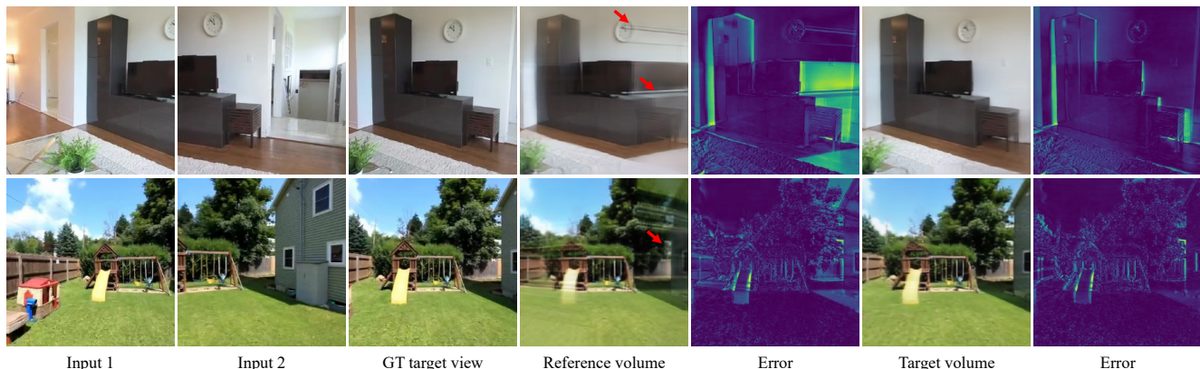
Figure 5. Our target view volume vs. reference (first image) view volume. Constructing the volume at the pre-defined reference view space might miss relevant information (e.g., red arrows regions) in other views since such information could be far away from the the reference view’s epipolar lines and thus hard to be sampled. In contrast, we construct the volume in the target view, which more effectively aggregates information from all input views and thus maximizes the information usage.
