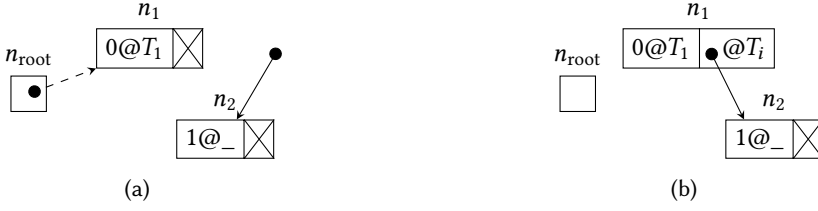
Fig. 5. Installing an Rc reference to a zero-count node. (a) n_{root} initially points to n_1 . Thread 1 gets a Snapshot to n_1 , creates a new node n_2 (getting an Rc), and gets a Snapshot to n_2 . Thread 2 updates n_{root} to null, decrementing n_1 to zero at time T_1 . (b) Thread 1 installs the Rc reference to n_2 on n_1 at time T_i . When n_1 is destroyed, we want to know if n_2 can be immediately destroyed.
