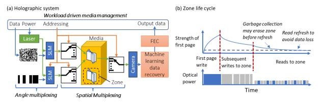
Fig. 1. (a) End-to-end holographic optical storage system, consisting of: media management, angle multiplexing within a single zone and spatial multiplexing across zones, with machine learning based decode. (b) Managed zone life cycle with optimized write and read energy profiles and refresh.
