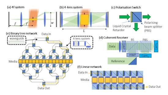
Fig. 2. Spatial multiplexing. (a) Typical 4f image relay. (b) 4-lens balanced image relay. (c) Fast polarization switch. (d) Coherent receiver (e) Low loss binary tree network. (f) Compact linear network.
