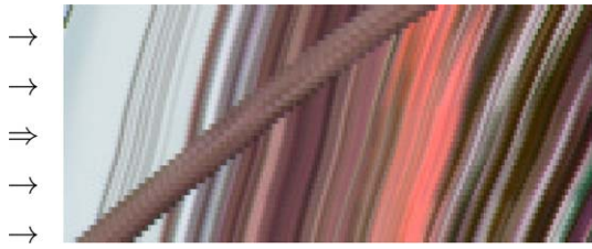
Figure 1. Slice through a motion stereo sequence spatio-temporal volume. A standard estimation algorithm only estimates the motion at the center frame ( \Rightarrow ), whereas our multi-view approach produces several additional estimates ( \rightarrow ). A layered motion model would use two (or more) layers to describe this motion, whereas a volumetric approach would assign one voxel to each “streak”.
