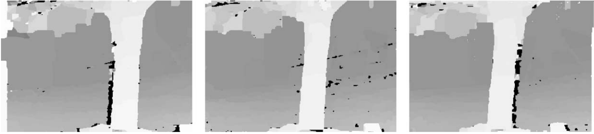
Figure 13. Effect of using the undefined label for 11-frame flower garden sequence (64 depth levels, no visibility terms, using best frames): (a) Reference image is 1st image, (b) Reference image is 6th image, (c) Reference image is 11th image. The undefined label is black, while the intensities for the rest are bumped up for visual clarity.
