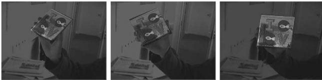
Fig. 16. Tracking with six degrees of freedom. These clips were generated by training an RVM displacement expert to work with six degrees of freedom in the affine similarity space. This approximately models the projection of a planar object undergoing out-of-plane rotations.
