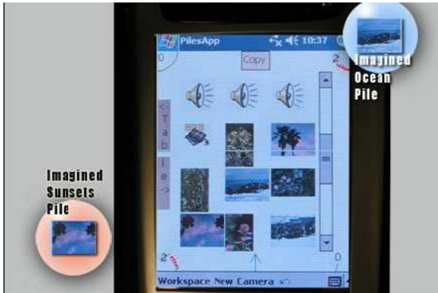
Figure 18: The PDA interface for Multi-User Piles Across Space. A “teleportation” zone to transfer piles to the table is located along the left-hand side. Dragging individual items or piles into this zone initiates a wireless file transfer to the table, where the items reappear.
