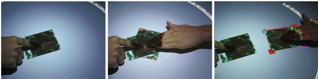
Figure 34: The “duplicate” policy automatically creates a second copy of a document that is simultaneously accessed by two people.
