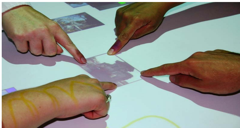
Figure 48: Four group members perform the “enlarge” gesture by simultaneously touching the corners of a single photo.
