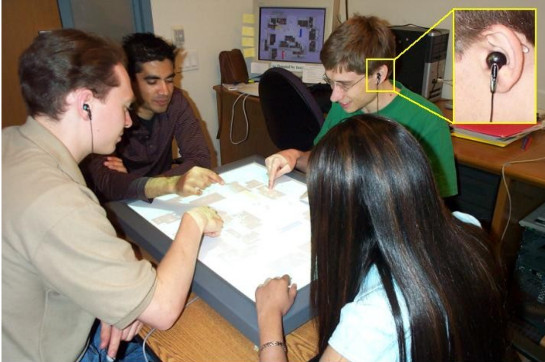
Figure 7: Four users sitting around a tabletop display can receive private information over their individual earbuds.
