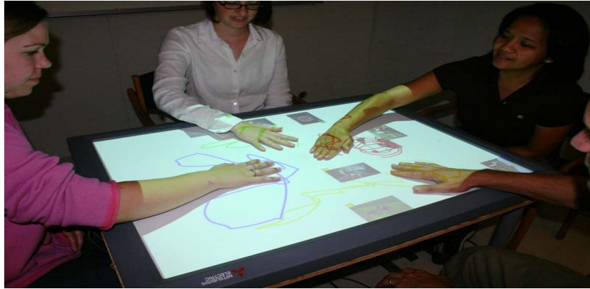
Figure 45: When all group members simultaneously “erase,” the “clear screen” action is invoked.
