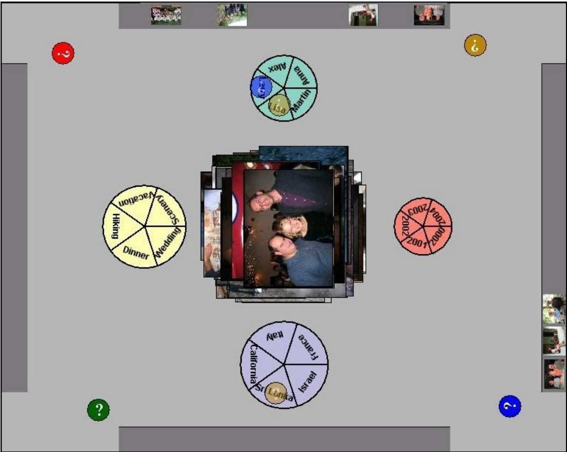
Figure 27: TeamSearch with parallel query tokens: each group member’s tokens (distinguished by color) form distinct queries.
