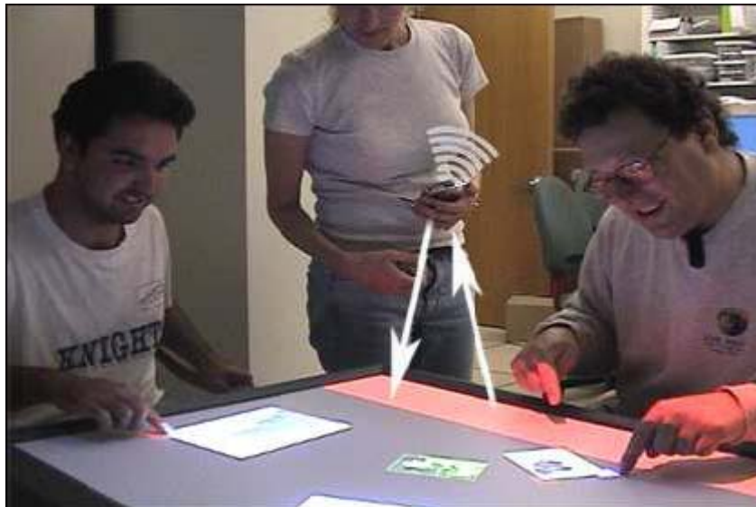
Figure 17: Three users by the tabletop display. The center user has transferred content from her PDA to the table to share with her coworkers.
