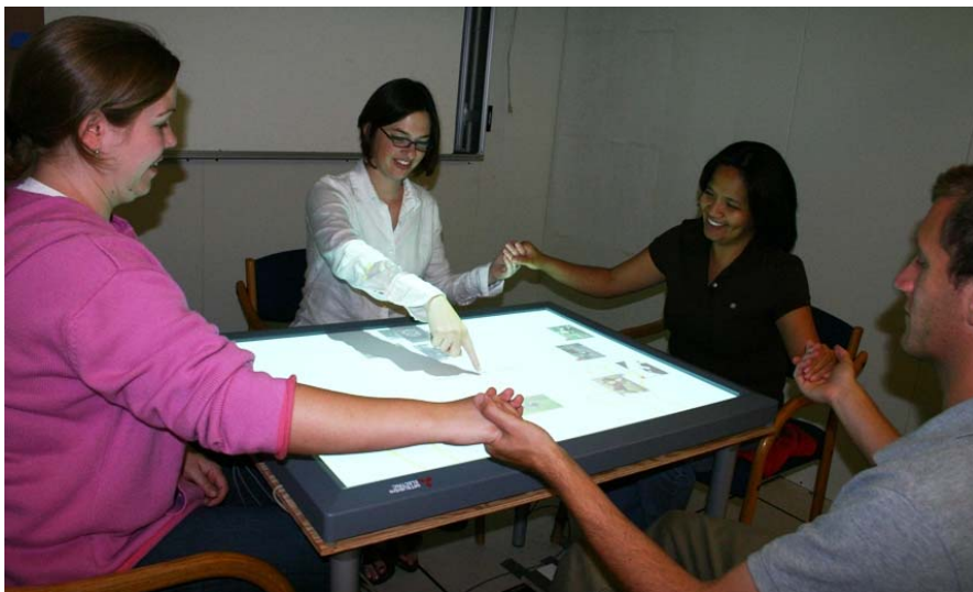
Figure 52: Group members form a chain by holding hands, and one user touches the table in order to exit CollabDraw.
