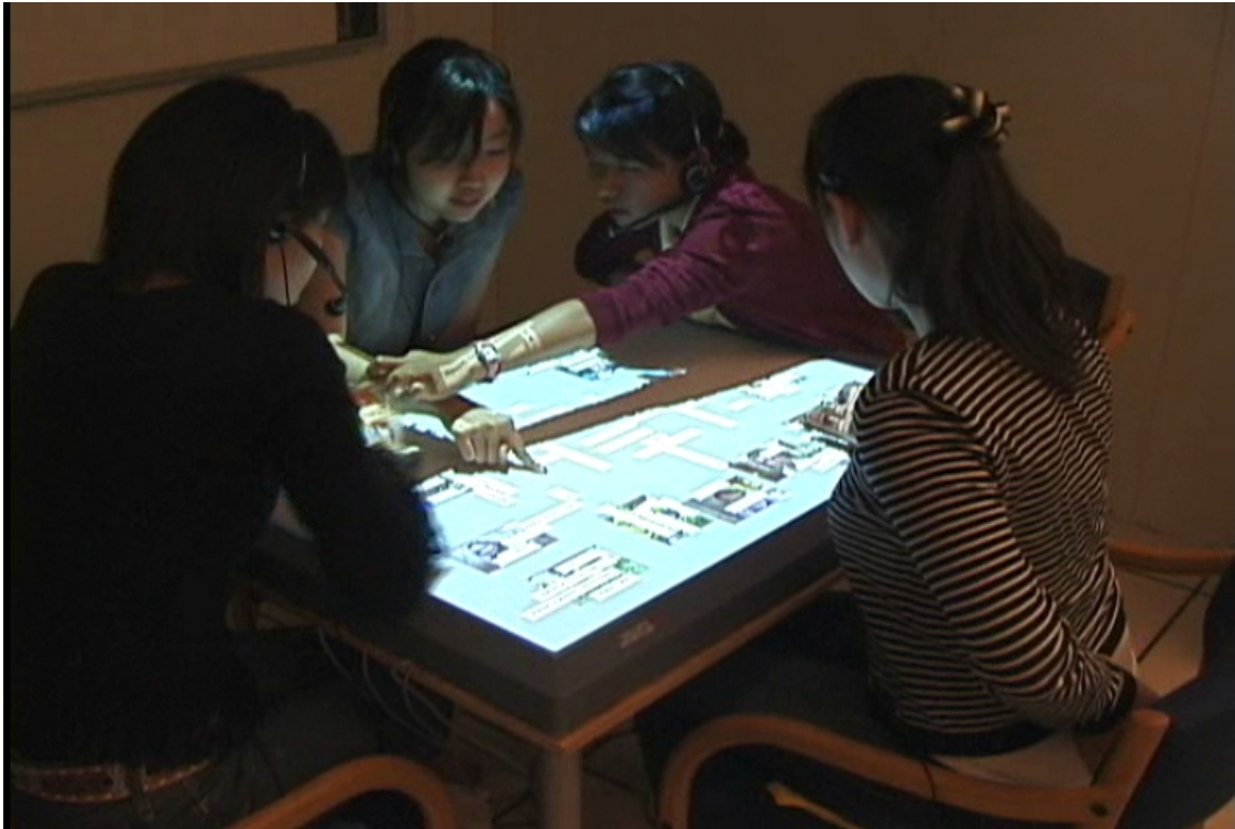
Figure 38: Four students sit around a touch-sensitive DiamondTouch table, working together to match pictures with words in a foreign language, using the MatchingTable software.
