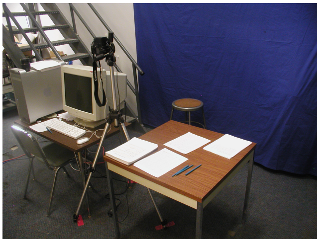
Figure 2. Setup for the high resolution image capture. Subjects were seated in front of a blue background and recorded using a Canon EOS 10D camera with a Macro Ring Lite MR-14EX ring flash.
