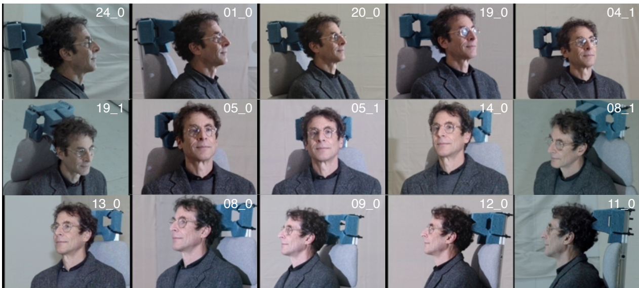
Figure 7. Montage of all 15 cameras views in the CMU Multi-PIE database, shown with frontal flash illumination. 13 of the 15 cameras were located at head height with two additional cameras mounted higher up to obtain views typically encountered in surveillance applications. The camera labels are shown in each image (see Figure 3).
