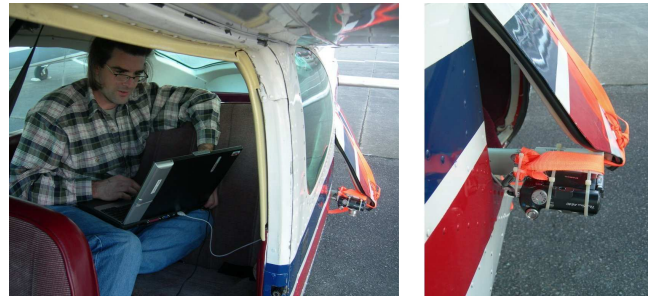
Figure 2: Our operation: a consumer camera zip-tied to a PVC pipe protruding from a hand-flown Cessna 177.
