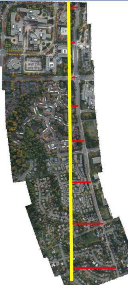
Figure 6: A straight road, captured with 12 aerial photographs and mosaicked using an image stitcher. Without geographic constraints, the road appears to curve.
