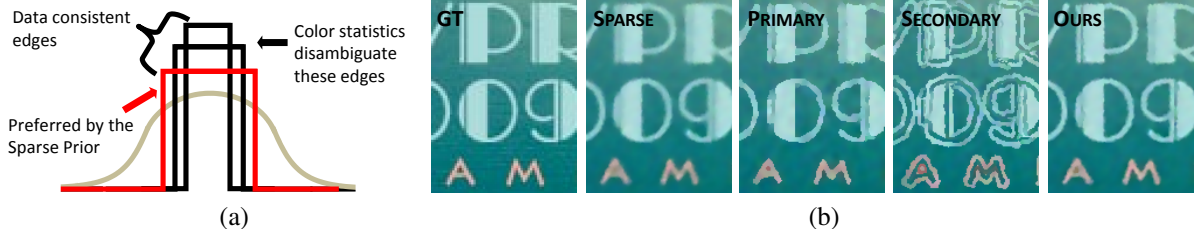
Figure 2: (a) Many sharp edges can blur to match an observed blurred (and potentially noisy) edge (in tan). The sparse prior always prefers the smallest intensity gradient that is consistent with the observation (in red). Our method picks the edge that is more likely given the dominant primary and secondary colors in the pixel’s neighborhood. (b) The thin blue areas between the white letters are deconvolved to a mid-level blue with the sparse prior. With our method the blue spaces are more distinct and edges are sharper.
