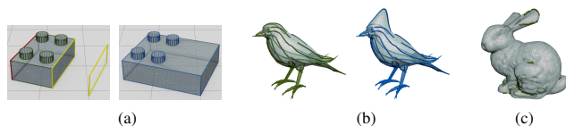
Figure 9: Limitations: (a) Spurious wires on the cylindrical parts cause over-constraining, and these parts no longer move during editing. (b) We may fail to detect meaningful relationships between the wires, resulting in limited effects when editing. (c) Our simple wire extraction procedure may fail to detect any wires; the editing framework then simply reduces to detail-preserving deformation.
