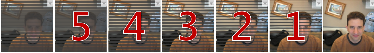
Figure 2: The countdown timer and the animated opening of window blinds inform the user that the application will soon be able to access a video stream—unless he disables it first.
