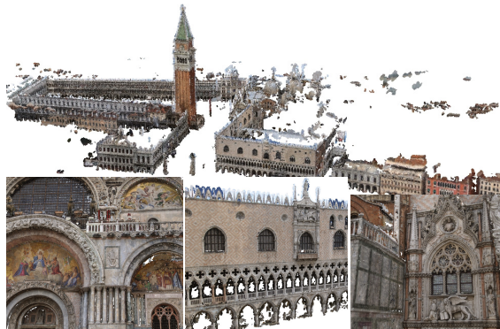
Figure 1. Our dense reconstruction of Piazza San Marco (Venice) from 13,703 images with 27,707,825 reconstructed MVS points (further upsampled x9 for high quality point-based rendering).
