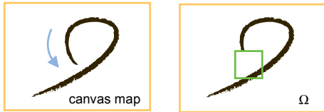
Figure 10: The canvas snapshot buffer \Omega is all up-to-date except for the area covered by the pickup map, preventing repeated resampling and the attending blurring.
