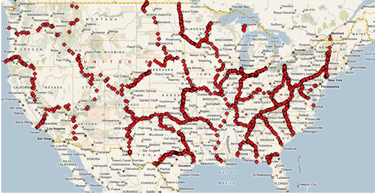
Figure 1: Example for a partition generated by PUNCH. The input is the road network of the US, taken from [7], having 24 million nodes and 29.1 million edges. We set U (the maximum cell size) to 1 million. The number of resulting cut edges is 1493 and the number of cells obtained is 30.
