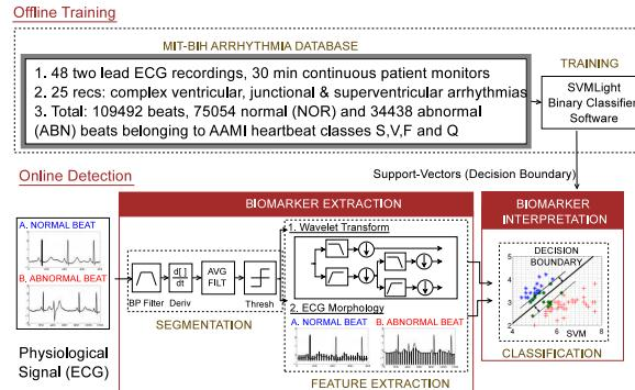
**Figure 1: The structure of data-driven biomedical detection algorithms includes (1) offline training, (2) online detection (employing biomarker extraction & biomarker interpretation).**
