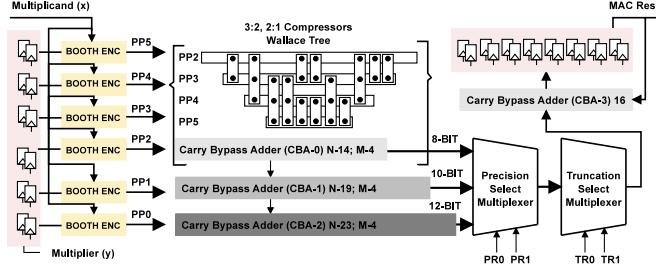
**Figure 9: The variable-precision MAC unit.** The partial product additions can be terminated at CBA-0/1/2 to scale the precision for 8/10/12 bit inputs. The figure also shows energy savings of 17.6% while scaling the precision from 12 to 8 bits.
