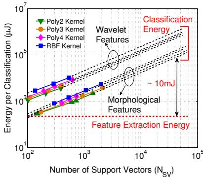
**Figure 2: Classification energy scales with  $N_{SV}$  and thus dominates that of feature extraction.**
