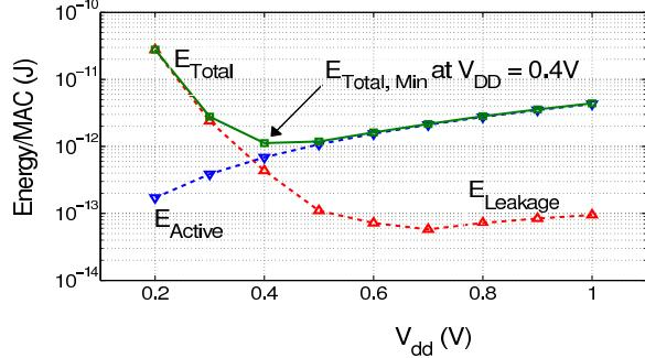
**Figure 6:** The active-switching and leakage energy profiles for a MAC unit with the min. total energy occurring at  $V_{dd} = 0.4$  V.
